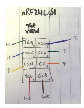
The pins on board need to go to specific digital output signals on the arduino.
